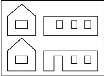
Firstly plot out the different elements of your design that will make up the 3 dimensional model. This can be drawn on computer and printed out or by hand onto paper which is then photo mounted onto the foam board. Alternatively the design can be drawn directly onto the foam board. Drawing the design on computer easily allows extra detail to be added such as brick patterns.
