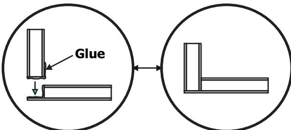
When you cut out the elevations on one side of the joint cut away the thickness of the board but only cut through the top board and the foam leaving the bottom board uncut. Then glue together as before. This will give a greater gluing area and a concealed joint. If you are using this method an allowance needs to be made on the elevations.
